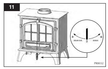
• Minimum position for burning solid fuel, Diagram 11
